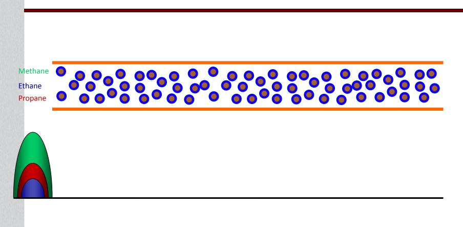
One at a time, each component leaves the Column and heads to the Detector for measurement
