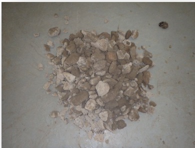
Crushed concrete residue
