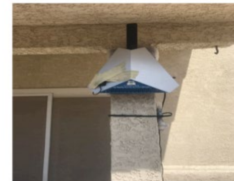
Figure 4. Illustration of (a) NFRM and (b) SCI 608 air quality monitors at the SVHS and Darby site, respectively.
