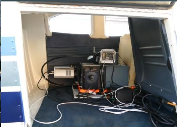
MAX-DOAS Spectrometer on the back seat
