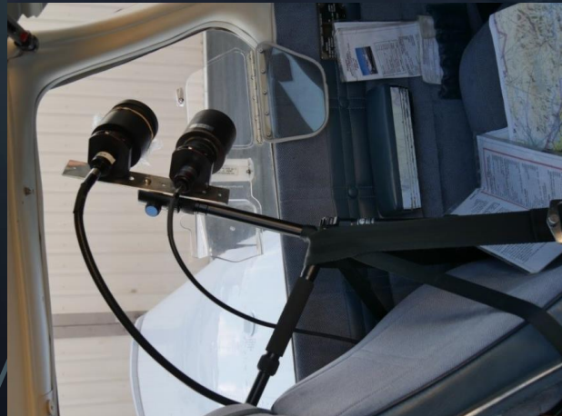
MAX-DOAS Telescope looking out of pilot's window
